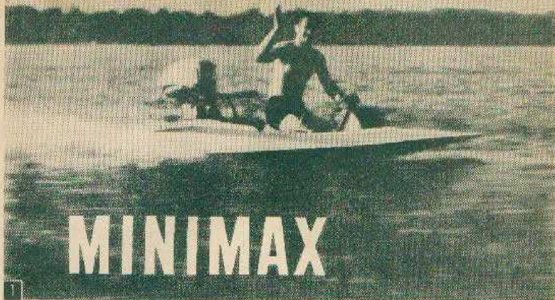
With a 10 hp outboard motor Minimax skims across the water at 35 mph. Air compartments make it unsinkable.
