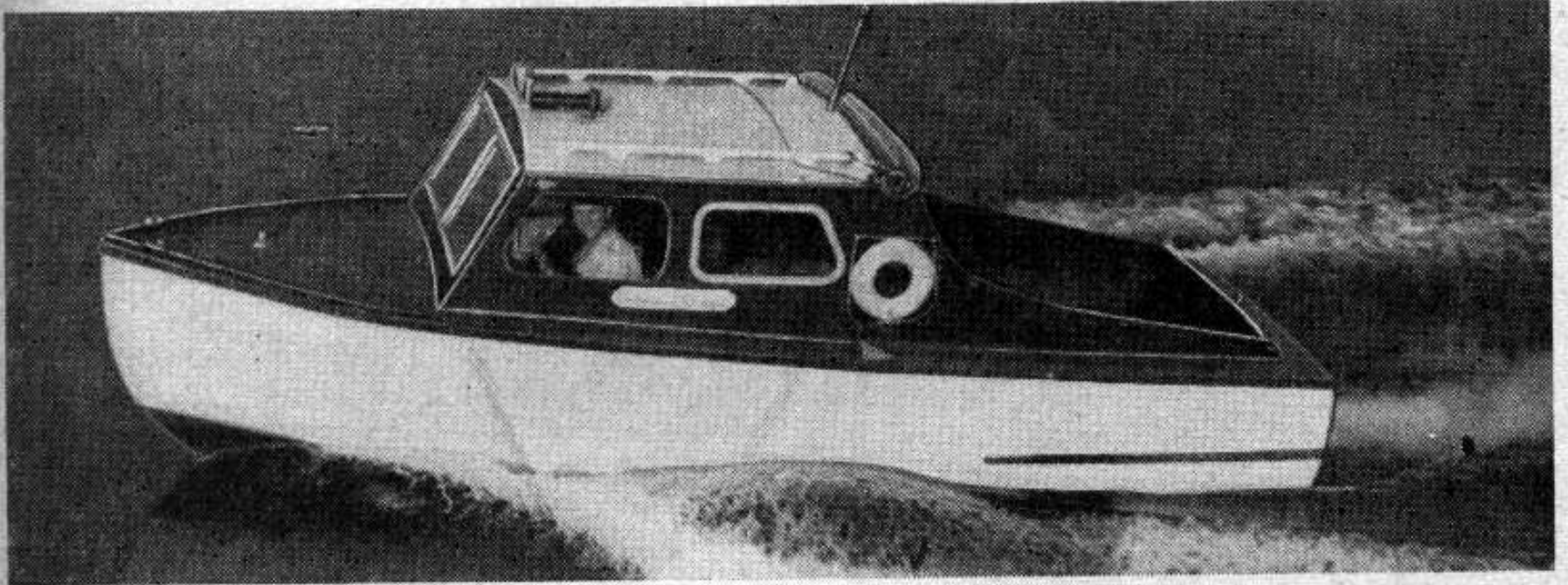
Nancy Jane as shown above was built by Charles Sears of Buffalo, New York, using hand tools exclusively and without outside help. He powered it with a 90 hp Dodge conversion which could turn a 12x13 prop at 3200.
