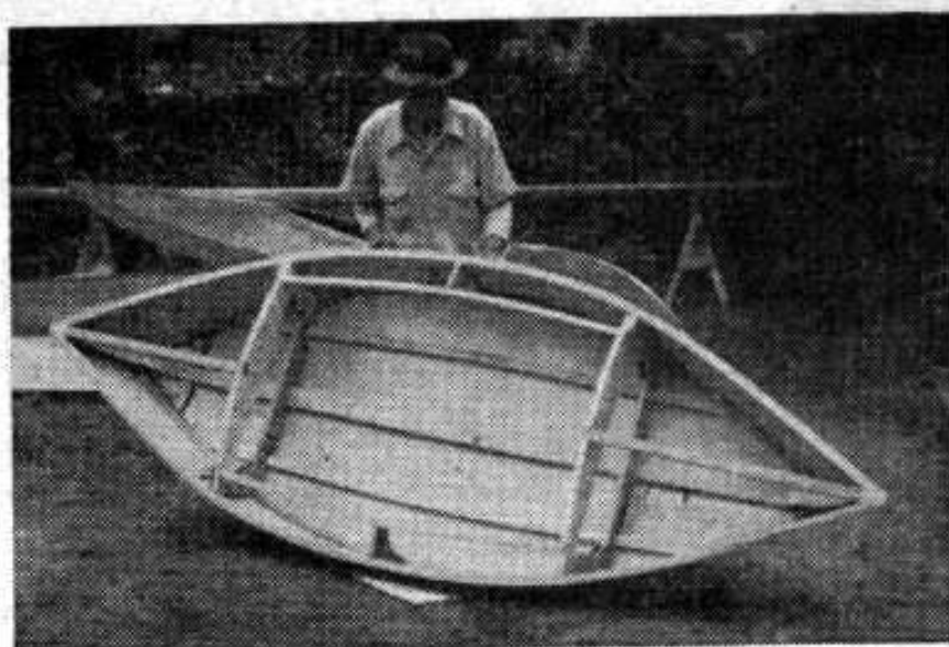
Fig. 7. Deck beams, carlins, side cockpit knee and deck battens in place.
