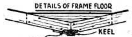
CUT NOTCHES ON EACH SIDE OF KEEL FOR LIMBER HOLES TO DRAIN
