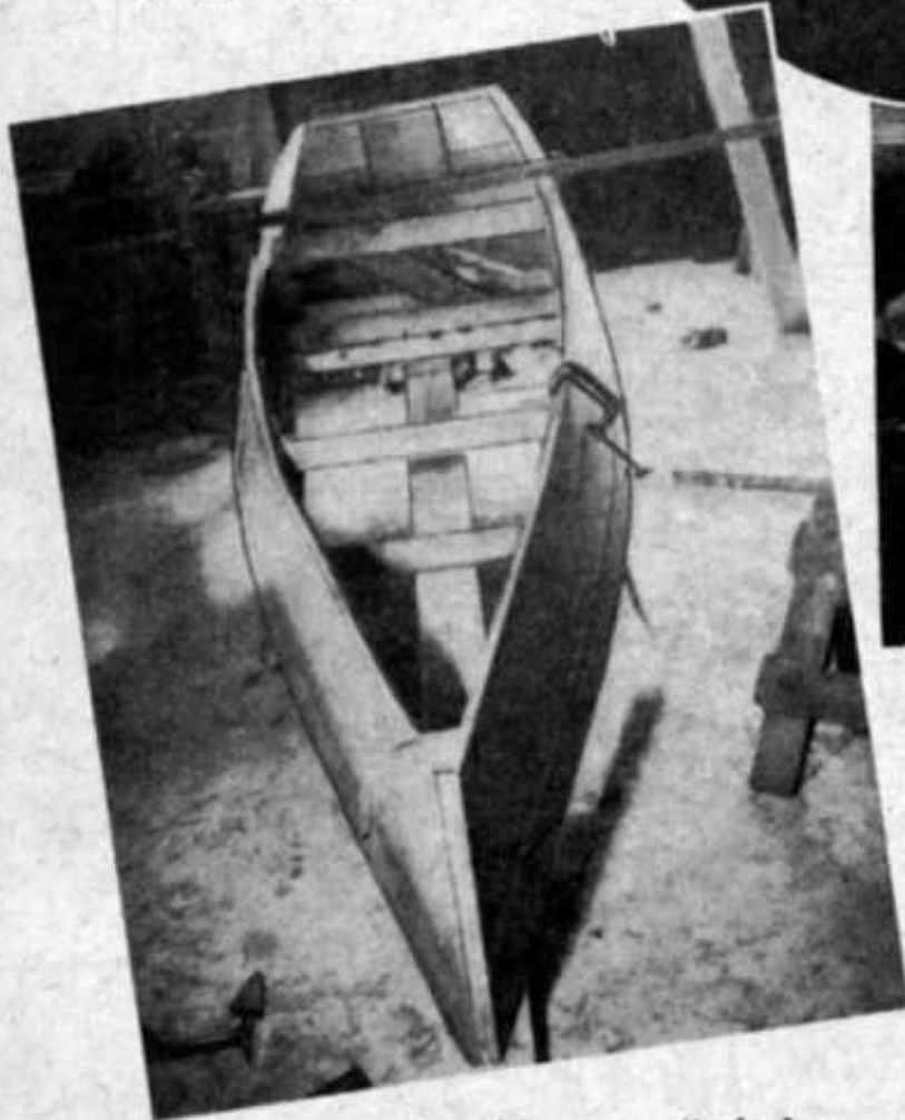
Side planking before chines are attached.
