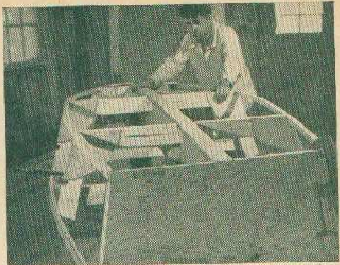
Stern view of completed framework with clamps in place.
